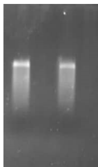
Figure 3: Transcribed HCV RNA from in-vitro transcription system on gel electrophoresis. The samples were diluted to one-twentieth in both lines.
